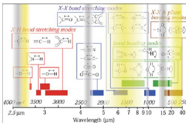
**Figure 7** – The 2.5-40  $\mu\text{m}$  spectral range is ideal for detecting and identifying both gas and solid state molecules. This region can only be fully observed from space – the shaded sections represent regions blocked by atmospheric H<sub>2</sub>O (yellow), and O<sub>3</sub> and CO<sub>2</sub> (gray)
