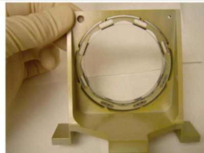
**Figure 12** – ABE-ASTID beamsplitter development (bottom) demonstrates required channel separation for ASPIRE moderate resolution spectrometer (top).
