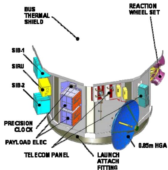
**Figure 14 – ASPIRE spacecraft bus layout with externally-mounted components.**
