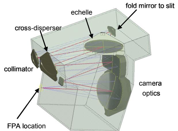
**Figure 11** – The ASPIRE Spectrometer configuration, which is replicated for each of the spectrometer arms
