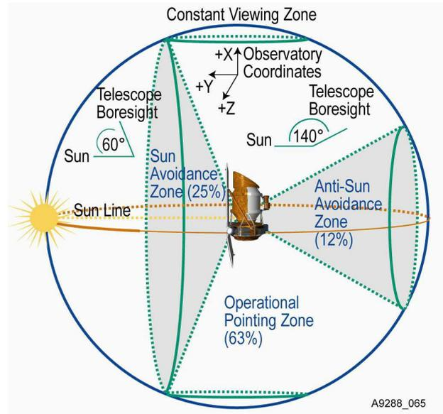
**Figure 8 – The ASPIRE Observatory has a instantaneous viewing annulus at any given time which sweeps across the entire sky every 6 months**
