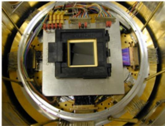
**Figure 13** – First high performance low temperature 1024 x 1024 Si:As IBC SCA under test at NASA Ames Research Center.
